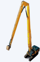
Demolition Equipment (38~90 tons)
