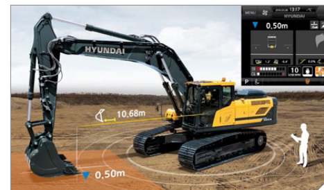
An example of using the Hi ASSIST technology for real-time surveying and automatic control
